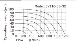
The data in flow rate chart are obtained from AirTAC lab.
